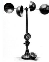
THE ROBINSON ANEMOMETER.
